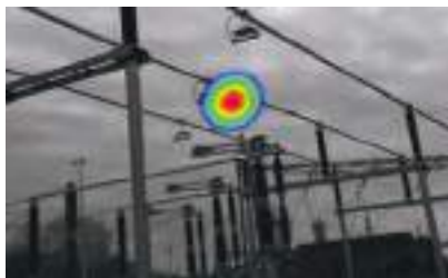
Built with 124 microphones, the Si124 produces a precise acoustic image that visually displays ultrasonic information, even in loud industrial environments.
