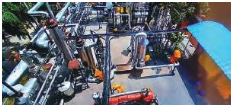
Photograph shows Thermax's 125-tpd pilot plant at Vadodara in Gujarat that produces hydrogen through gasification of woody biomass.
